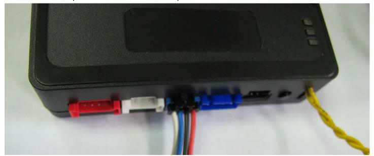
Or Cut the ATOM supplied connector with a knife as shown:
